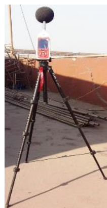
Fig .4.5: Sound level meter (Optimus, G066918, CR:162C) installed at the construction site
