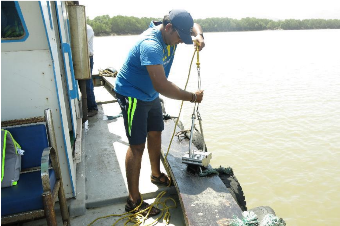
Fig. 4.7: Collection of bulk sediments using Van Veen Sediment Grab
